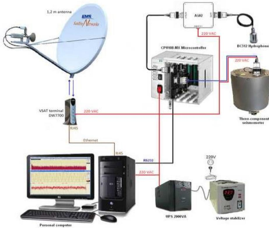
**Fig. 2.** Diagram of the station
