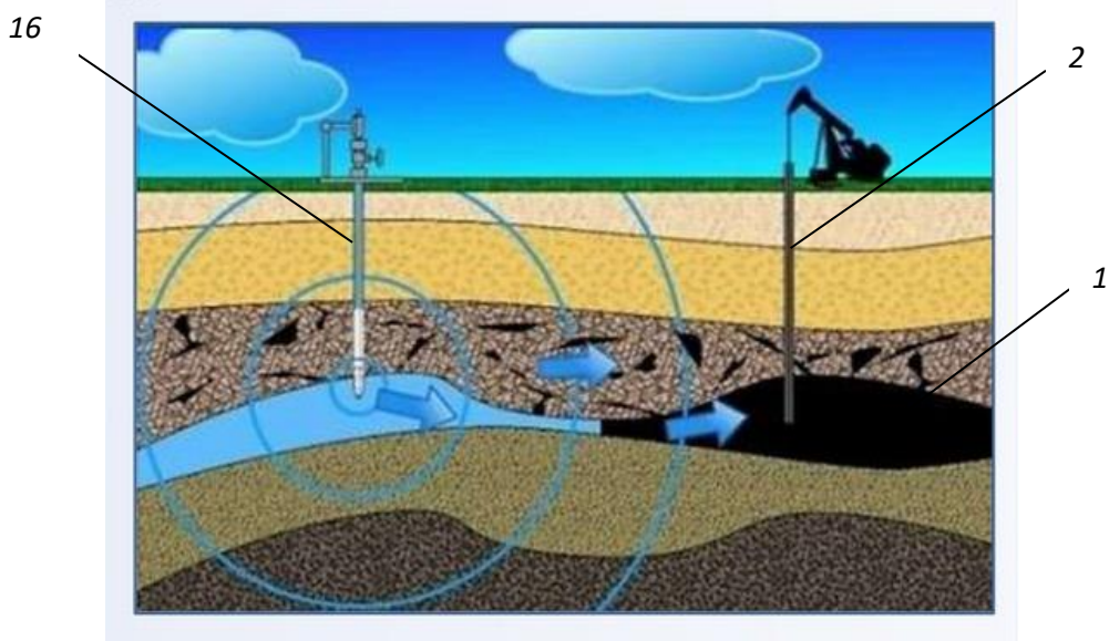
Fig. 1. Typical flow chart for oil production process in the late stage of field development.
