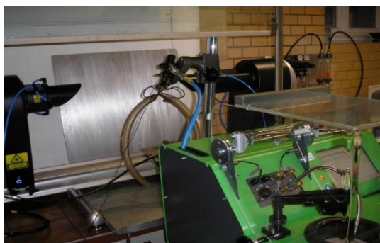
Fig. 2. A test station for determination of fuel drop diameter distribution
